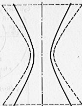
Fig. 8 Hyperboloid generated with lines of interference appearing as a hyperbola.
