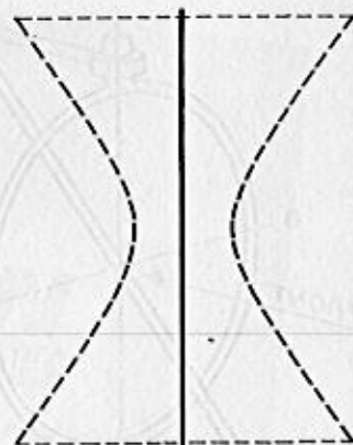
Fig. 6 Hyperboloid generated with line of interference as its axis.
