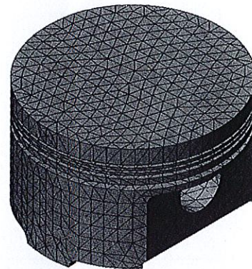
Figure 6 A Mesh is Generated Over the Solid Model for the FEA Study
