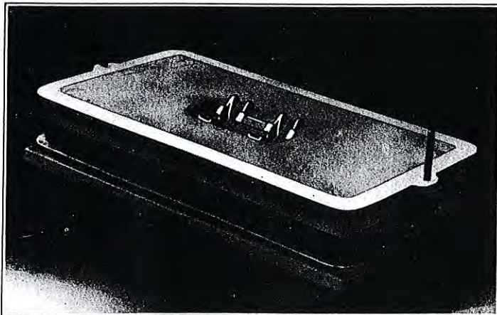
Pattern in position showing mold parted down.
